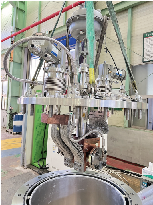
Fig. 2. The liquid hydrogen valve within the vacuum chamber
