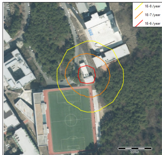
Fig. 11. IR contour of facility with mitigation
