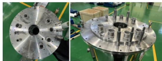
Fig. 3. Upper flange of LH<sub>2</sub> liquefier
