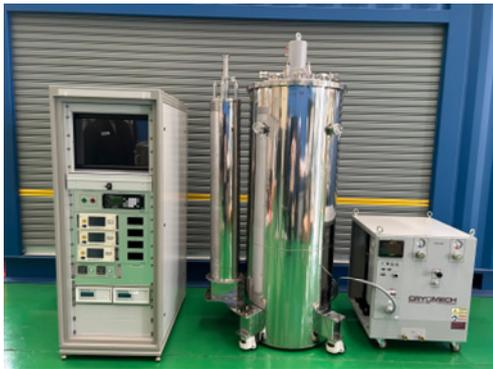
Fig. 6. Fabricated LH<sub>2</sub> liquefier
