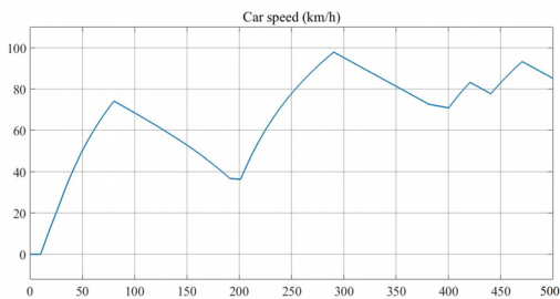
Fig. 3. Curb weight vehicle speed with accelerator load profile input
