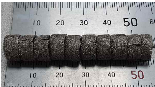
Fig. 2. Nickel foam cup for holding catalyst in multilayer cup structure (MLCS)
