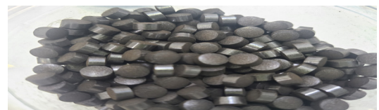
Fig. 1. Cu/ZnO/Al 2 O 3 DME steam reforming catalyst
