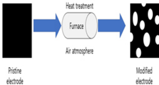
Fig. 2. The activation process of carbon felt
