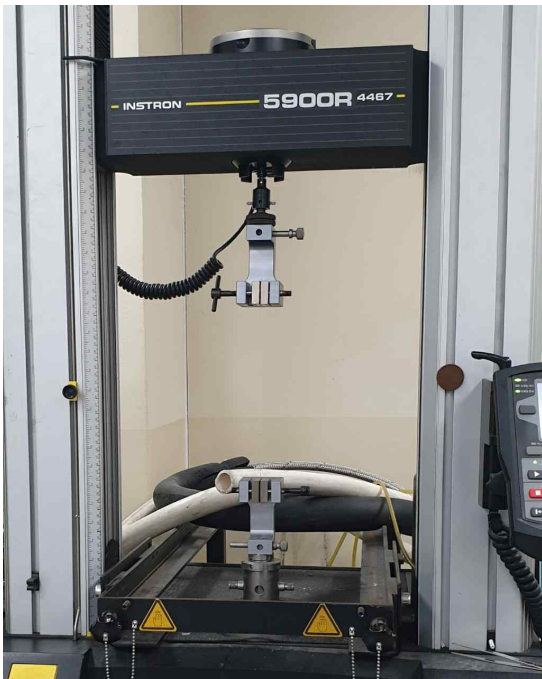
Fig. 2. Tensile testing apparatus for specimens of polymer electrolyte membrane
