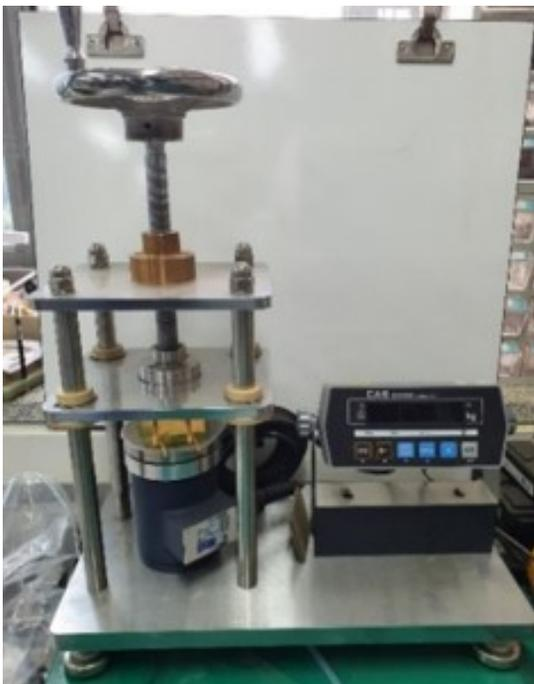
Fig. 2. Picture of the contact resistance test setup
