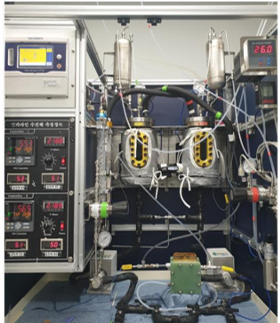
Fig. 4. In situ water electrolysis cell test station
