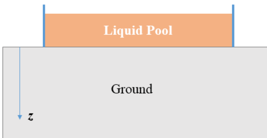
Fig. 4. Vaporization of non-spreading pool on ground
