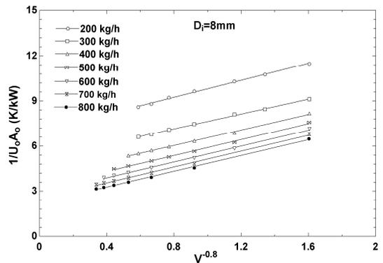
Fig. 4. Wilson plot for tube diameter of  $D_i=8.0$  mm
