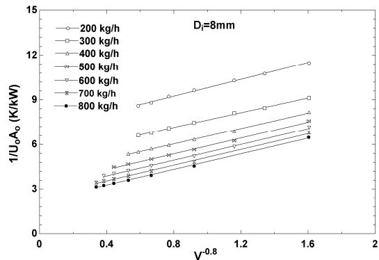
Fig. 4. Wilson plot for tube diameter of  $Di=8.0$  mm
