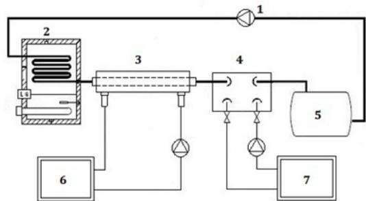
Fig. 1. Schematic diagram of experimental facility (1. Refrigerant pump, 2. Pre-heater, 3. Test section, 4. Plate heat exchanger, 5. Receiver tank, 6&7. Chillers)
