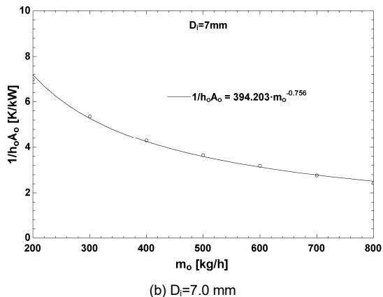
Fig. 6. Heat transfer coefficient for annular side vs. mass flow rate (a)  $D_i=8 \text{ mm}$ , (b)  $D_i=7 \text{ mm}$
