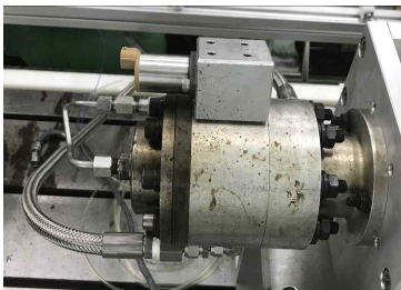
Fig. 1. Wobble plate type high pressure fuel pump used in experiment
