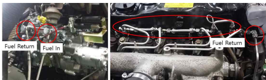
Fig. 2. Fuel system of test engine
