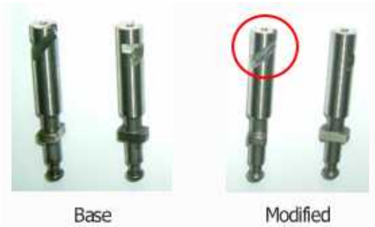
Fig. 3. Modified plunger of DME high pressure pump
