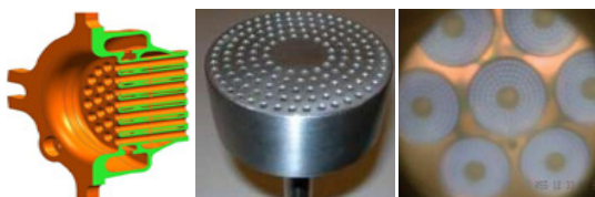
Fig. 10. Multi tube mixer of GE 6)
