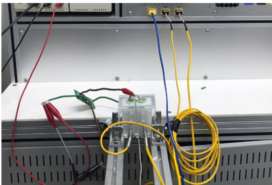
Fig. 1. Picture of the experimental system for the Li-ion battery with PCM-based cooling
